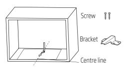
3. Remove the bottom cabinet template and fix the bracket with screw.
